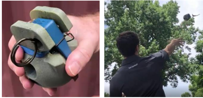
The M67 Frag Sim Grenade (left photo) has all the real components that a soldier interfaces with – Pull Pin, Spoon, & Safety Clip. An employee throws the Sim Grenade and the spoon fly-off is visible (right photo) indicating that the fuse has begun its 5 second delay.
