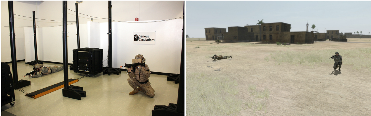
Body and tracking translates position data to virtual avatar in real time
