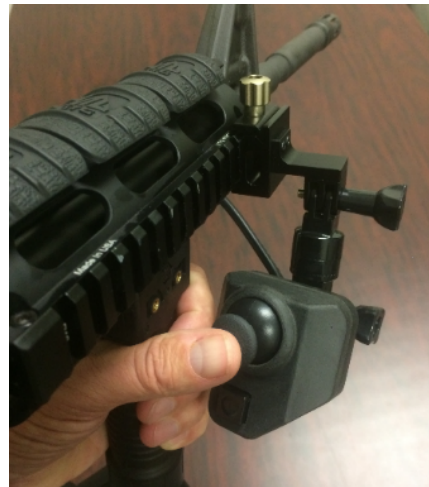
Natural positioning for interfacing Thumbstick and menu buttons for a variety of thumb sizes
