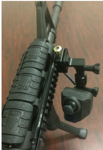
Real weapon mounted Thumbstick Controller with ergonomic adjuster
