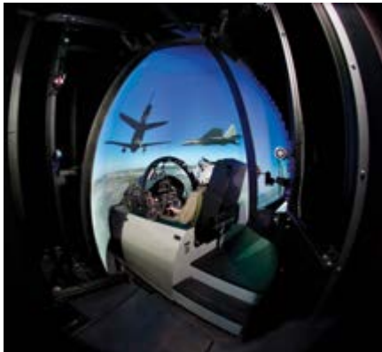
Boeing has launched the latest version of its CRVS to provide 20/20 acuity throughout a 360° FoV using JVC D-ILA projectors. (Photo: Boeing)
