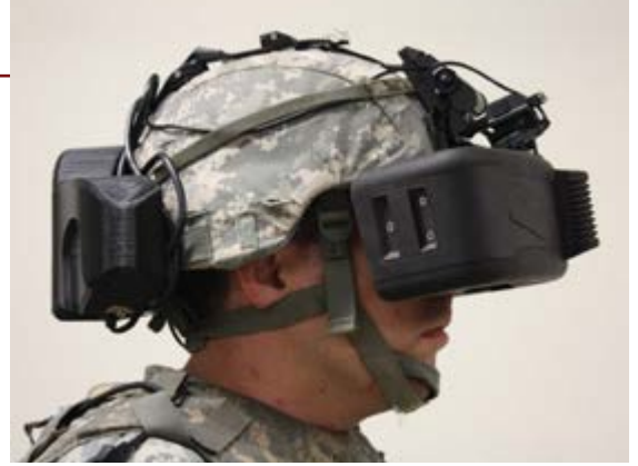
Serious Simulations' 130° horizontal FoV HMD can be used to upgrade a number of different types of simulators, from door gunner trainers to dismounted infantry devices. (Photo: Serious Simulations)
